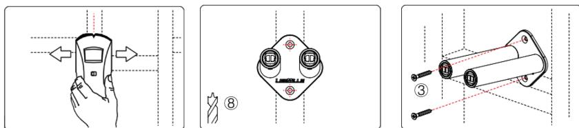
**STEP 1** Use a stud finder to locate and mark the location of the existing studs in the wall.
