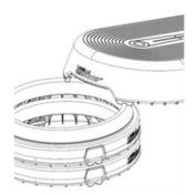
**Horizontal Use** - A maximum of 6 risers may be used under the SMARTSTEP deck at each end. Follow the assembly instructions when attaching risers.
